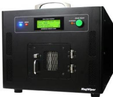
Most compact and Light weight. Simple and safe to operate. Metering and controls ensure complete erasure on each cycle. Portable due to small size and relatively light weight. Erasure zone capacity is one 3.5" HDD or eight 2.5" HDD. This plus a 15 second cycle time, continuous duty result in a high throughput of 240 3.5" HDD/hr or 1,920 2.5" HDD/hr.
